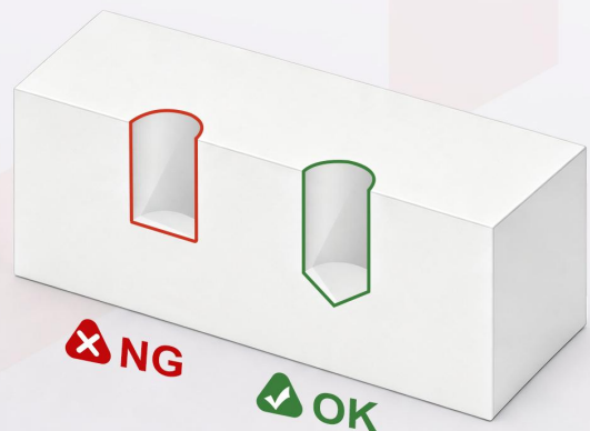
Figure 25 : Avoid Flat-Bottom Blind Holes
