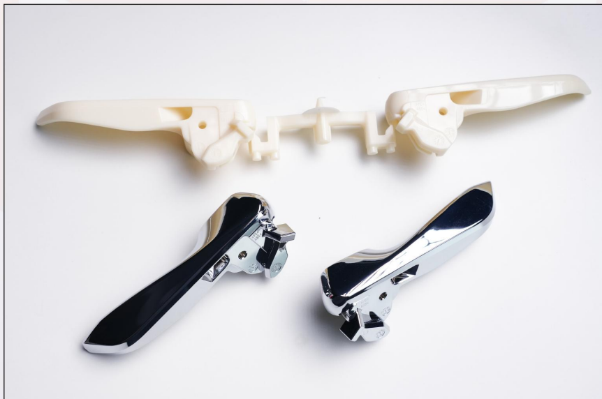
Figure 11. Plastic handle before and after electroplating.
